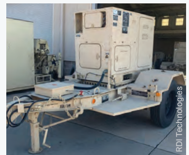
15 kW/400 HZ trailer-mounted Army tactical generator.
